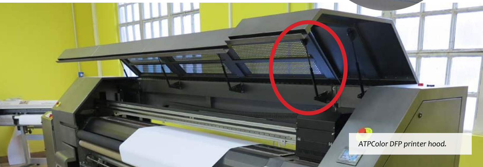
Close-up of the units from Starbulus, that raise the hoods
