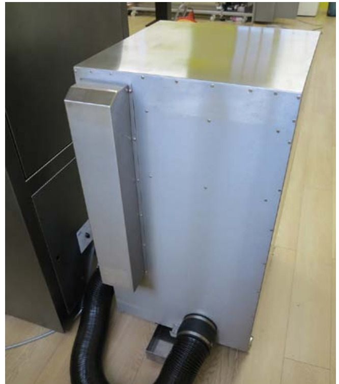
Views from the front (left) and back (right) of the printer's air cleaning system.
