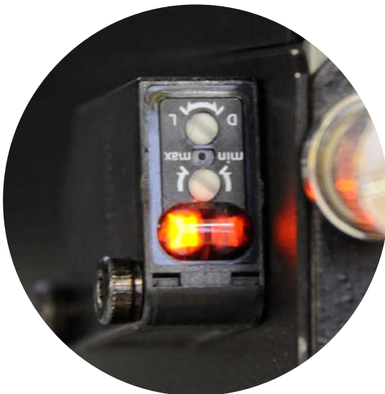
Printhead carriage and minimum and maximum head adjustment control.
