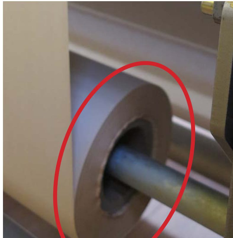
Media wound up on the back side of the printer, as you can see there is no skew.
